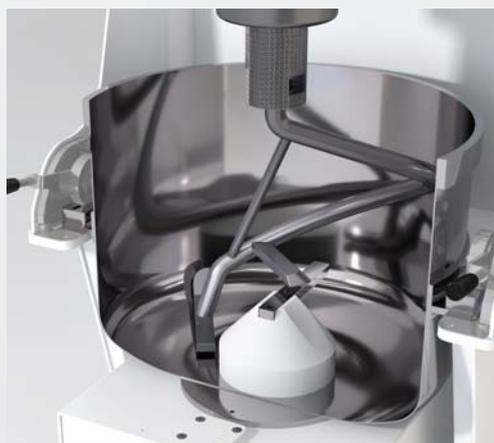
The tool pushes the dough that, obstructed by the cone-shaped protrusion, moves from the bottom to the top and breaks it apart to obtain perfect oxygenation without undue stress.
